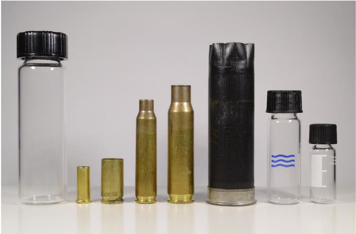
Figure 3-1 Comparison of various fired cartridge cases and headspace vials. From left to right: 14 mL vial; .22 LR; 9x19 mm; 5.56x45mm; 7.62x51mm; 12 gauge; 4 mL vial; 2 mL vial.
